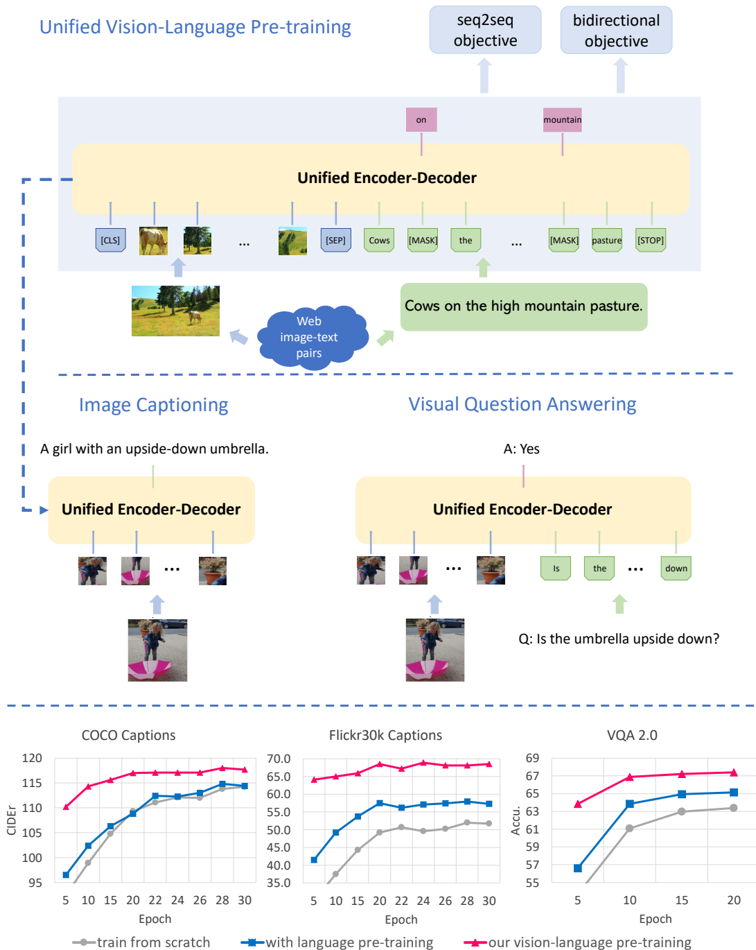
Figure 8.1: We propose a unified encoder-decoder model for general vision-language pre-training. The pre-trained model is then fine-tuned for image captioning and visual question answering. Thanks to our vision-language pre-training, both training speed and overall accuracy have been significantly improved on the downstream tasks compared to random initialization or language-only pre-training. All the results are evaluated on the validation set of the corresponding dataset.
