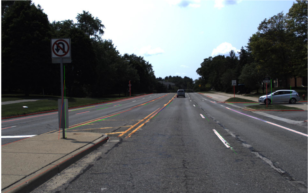
Figure 4.10: Data collected from an autonomous vehicle platform. This shows the estimate of our approach for three frames. Green is a line in 3D, red is a line detected in 2D, and blue shows an estimated association.
