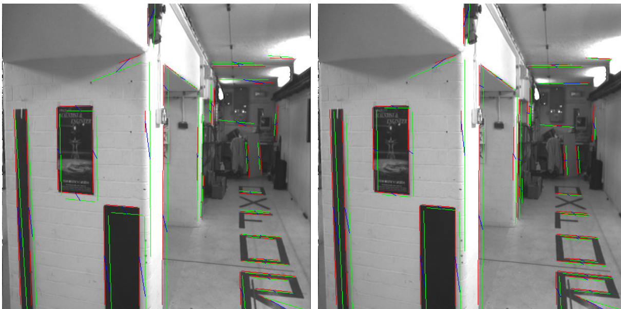
Figure 4.3: Comparison between the SVD approach presented by Přebyl et al. and our linear \ell_1 approach on the VGG Corridor sequence with known associations. Red lines are 2D lines from the image while green lines are 3D lines. From the the Corridor sequence.
