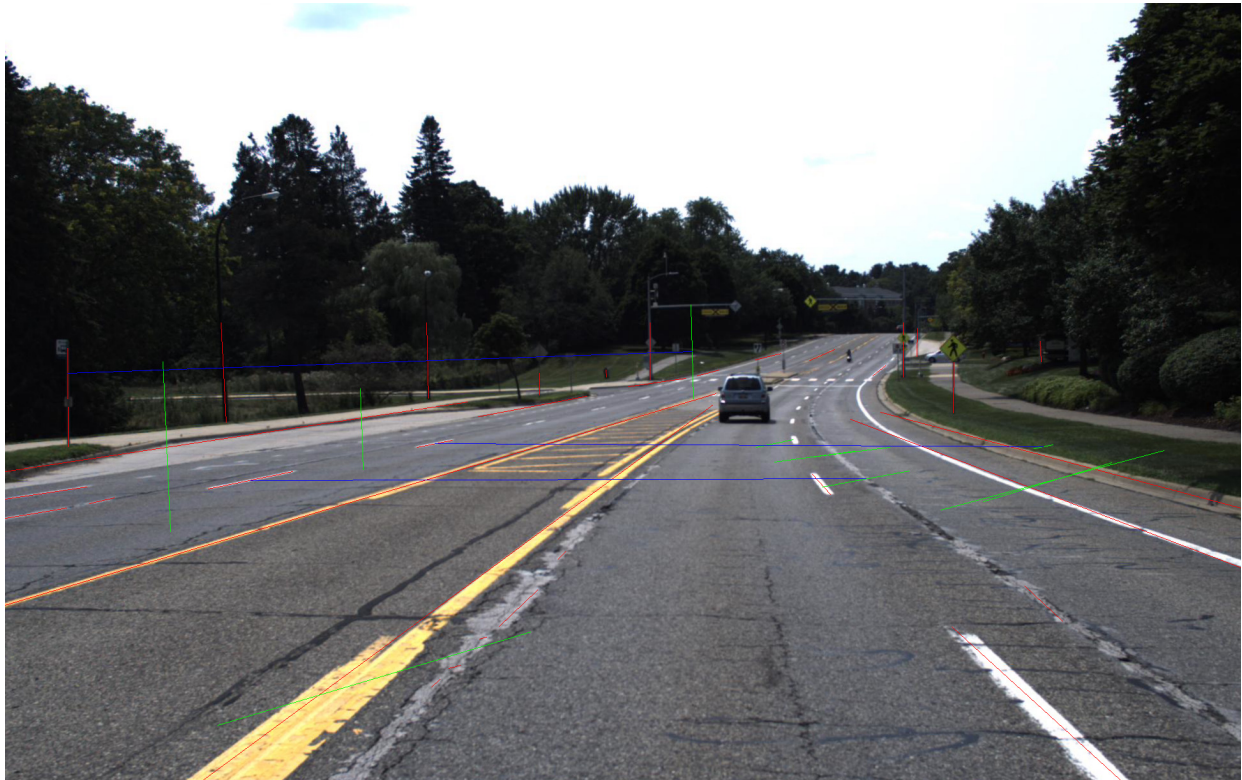
Figure 4.12: Data collected from an autonomous vehicle platform. This shows the estimate of our approach for three frames. Green is a line in 3D, red is a line detected in 2D, and blue shows an estimated association. This frame estimated an incorrect association and transformation, while the other two converged to the correct results.
