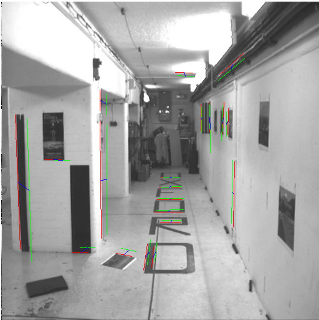
Figure 4.8: Results from the VGG dataset with unknown associations. Green represents 3D lines, red 2D lines, and blue connects the pairs association by our mixed-integer formulation.
