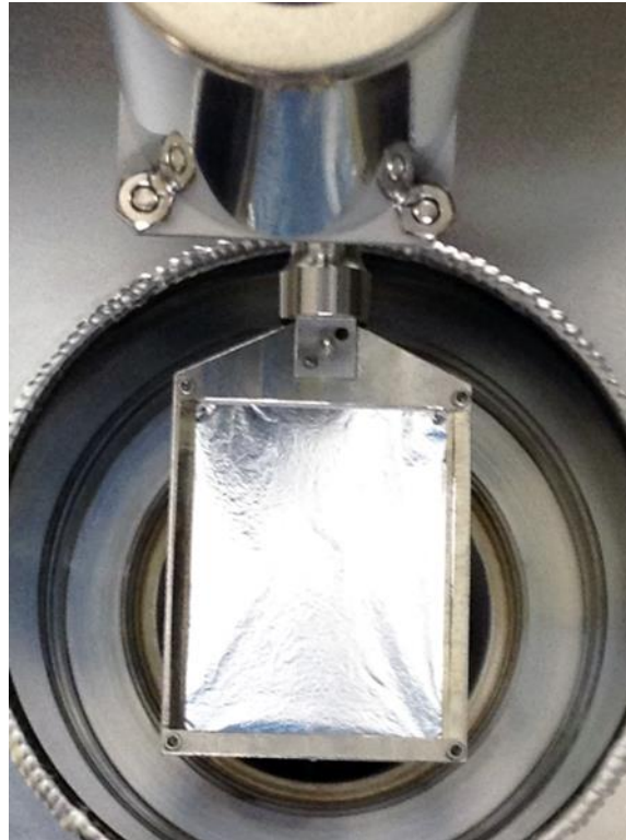
Figure B.4. The thin foil energy degrader used at the Michigan Ion Beam Laboratory for control of the implantation range of a light ion beam during multi-ion irradiation through foil rotation. The holder is shown with a 2.6 \mu\text{m} aluminum foil loaded and held taut by a crimp inside the holder frame.
