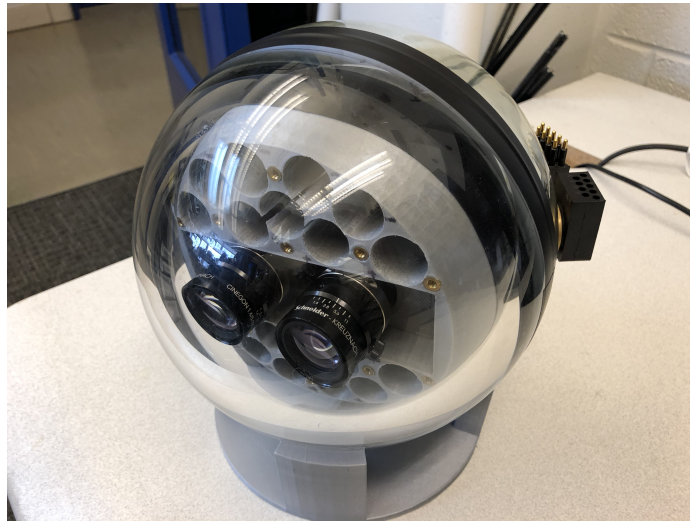
Figure 4.1: Stereo camera used for vehicle navigation. The position of the cameras is far from the center of the hemisphere, introducing significant distortion in the images.
