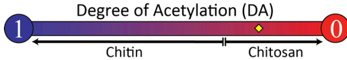
Figure 1.1 Spectrum of DA for chitin and chitosan. The yellow diamond represents DA = 0.28 for the chitosan used in Chapters 2 and 3.
