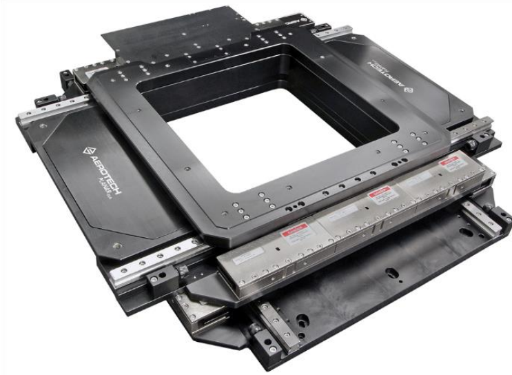
Figure 1.4 Planar NP stage guided by mechanical bearings [45].
