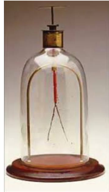
Figure 2-1: The gold-leaf electroscope.
