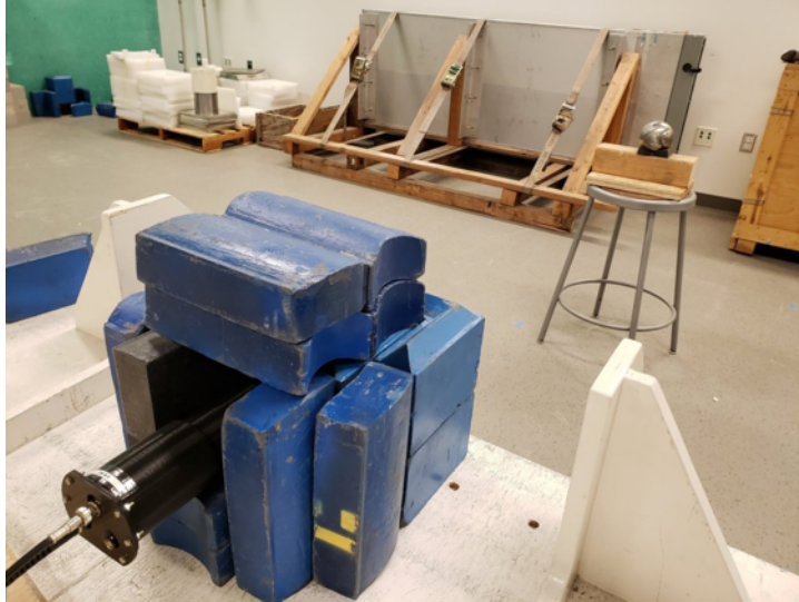
Figure 4.16: Stilbene detector housed in 10.16 cm lead cave, 1.7 m from tungsten target placed in beam center.
