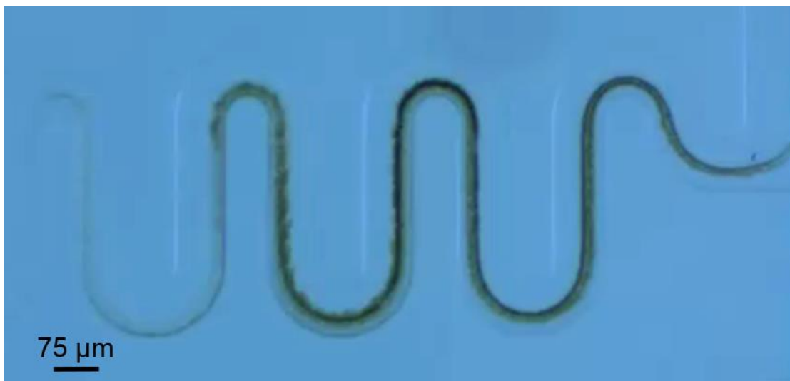
Figure 4-2: Precipitation at carbonate reagent addition junction in PDMS chip after 10 min of operation. Significant precipitation occurred at each of the three reagent addition junctions. Channel dimensions are 75 μm wide x 50 μm deep.
