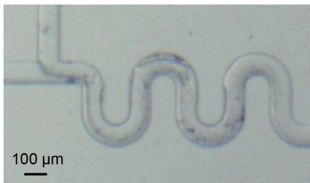
Figure 4-4: Precipitate formation at laminar interface of BzCl junction after on-chip derivatization of high concentration 25 compound standard mixture. Reagents were continuously flowed for the 2 hr duration of the experiment.
