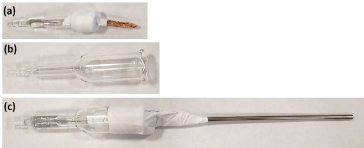
Figure 0-1 (a) Custom-made single-junction Ag/AgCl/KCl(sat.) reference electrode design. The AgCl-coated Ag wire is enclosed within a glass body filled with saturated KCl(aq) and separated from the electrolyte solution by a CoralPor® glass frit. (b) Glass frit which serves as the second junction. Custom-made glass body enclosed with a CoralPor® glass frit (c) Double-junction Ag/AgCl/KCl(sat.)/NaHCO 3 (0.1 M) reference electrode constructed by placing the single-junction Ag/AgCl/KCl(sat.) reference electrode into the glass body that serves as the second junction. The glass body is filled with electrolyte (resin-treated 0.1 M NaHCO 3 (aq) or 0.1 M H 2 SO 4 ) and separated from the electrolyte solution in the electrochemical cell by a CoralPor® glass frit. A stainless steel rod with an alligator clip is attached to the reference electrode during electrochemical measurements.
