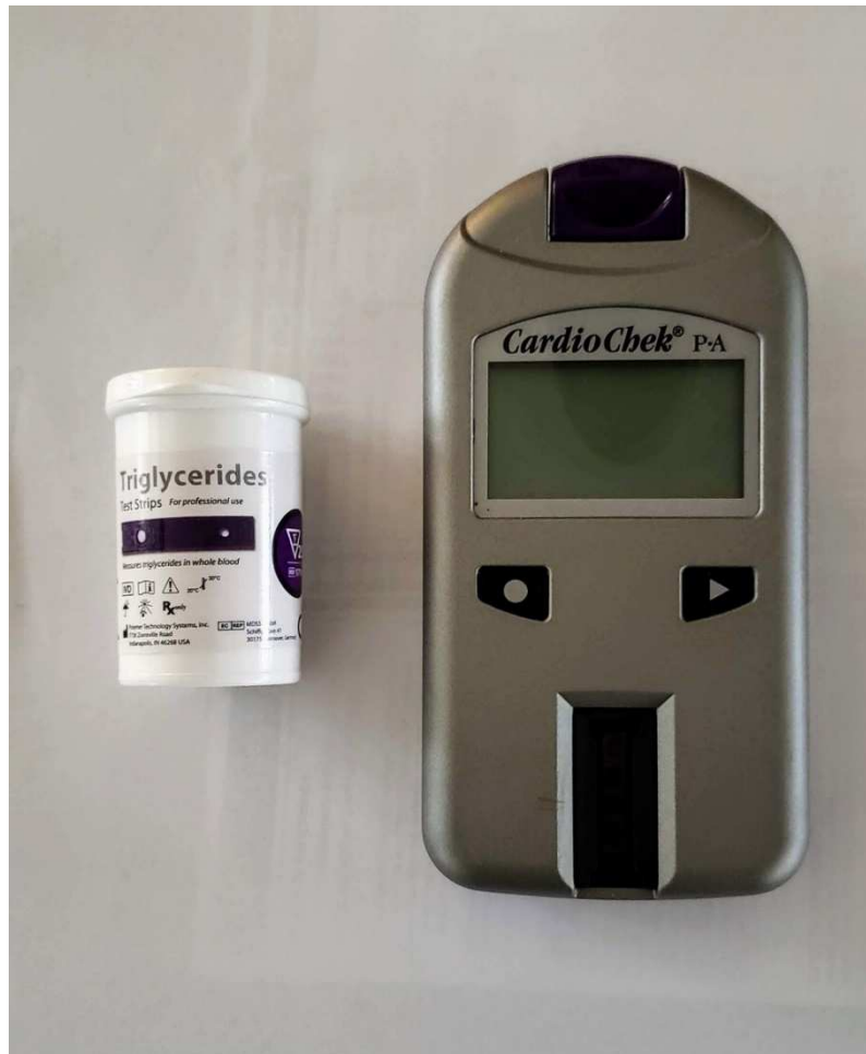
Figure 2.1: The CardioChek PA analyzer is a small handheld meter that is similar in size and ease of use as a glucometer. Paired with the triglyceride test strips, also pictured, allows it to be easily transported and used in a field setting.
