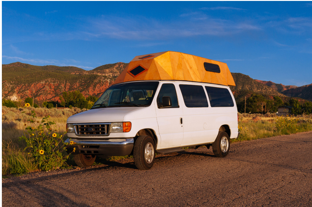
Right: Van with custom camper top, plywood on steel, August 24, 2018
