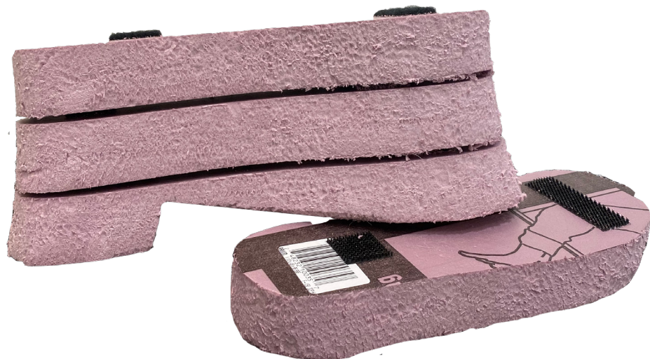
Right: Fig. 11, Image of Elevate-Ur-Shoes prototype prior to fiberglass coating.
