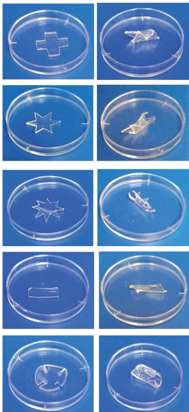
Figure 2. Left column: original shapes of AM-PEGDE films before they were placed on the surface of water. Right column: corresponding fabricated 3D structures obtained upon actuation by partial hydration of the gels for 1 min.
