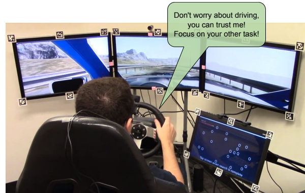
Fig. 1. An undertrusting driver is encouraged by the AV system simulator to focus on his non-driving-related task (NDRT), to increase his trust level. An analogous situation would take place if the driver overtrusted the AV's capabilities, with the system then demanding his attention to the driving task.
