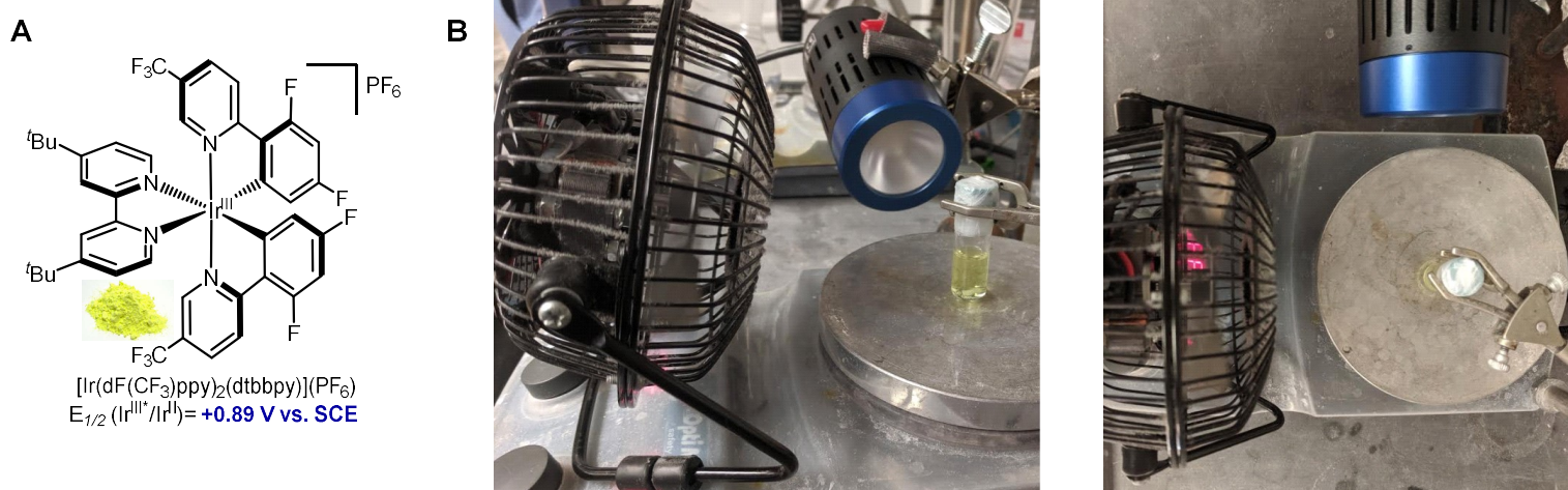
Figure 3.11. (A) Structure of photocatalyst; (B) Side and top view of reaction set up
