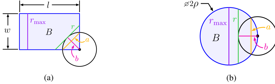
Figure 5.2: Examples (and visual proof) of the geometric quantities r_{\max} , r , b , and a , used to construct the discretized obstacle, for rectangular and circular robot bodies.
