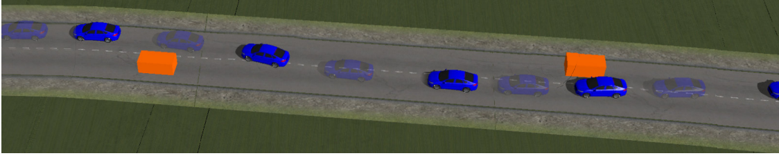
Figure 9.7: The Fusion passenger sedan using RTD to safely and autonomously plan and perform a double lane-change around static obstacles at 15 m/s (which is the speed limit of the road shown). The robot is simulated in the high-fidelity CarSim environment [Mec18], which models the robot’s hybrid powertrain and tire dynamics. Using RTD, the robot successfully navigated a 1 km test track, populated with random obstacles, with no collisions.
