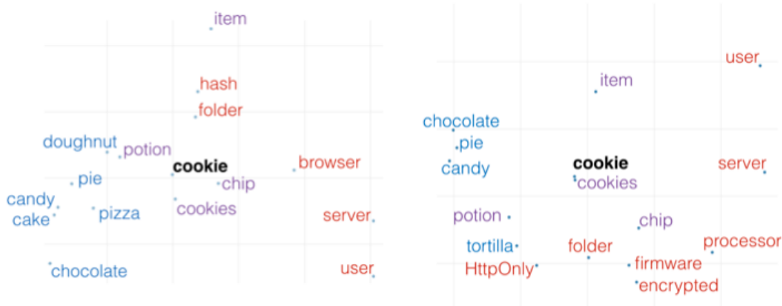
Figure 1.1: The word cookie and its fifteen nearest neighbors in two separate embedding spaces. Both spaces are trained on Wikipedia using word2vec; the random seed used to initialize word2vec varies between the two spaces. Here, we show the two-dimensional PCA [94, 58] projection of the embeddings (visualized partially with Parallax [89]). Nearest neighbors are chosen using cosine similarity distance. Food-related words are colored blue, technology-related words are colored red, and ambiguous words are colored purple.
