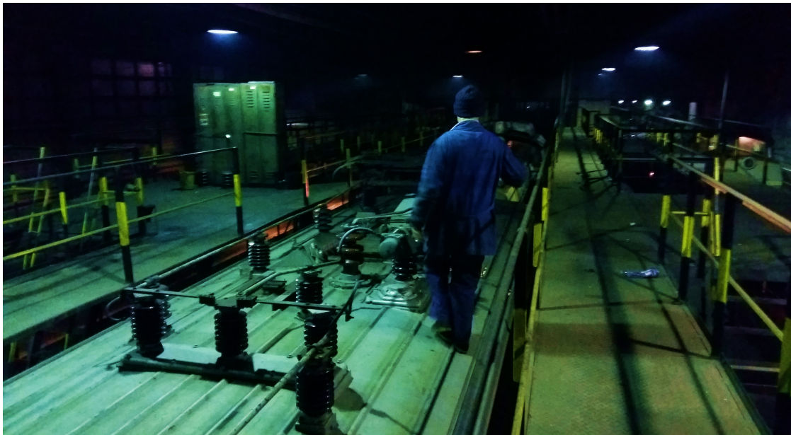
Illustration 44. Rooftop power system on a locomotive.
