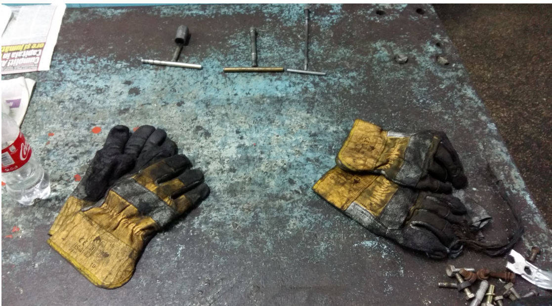
Illustration 35. T-shaped "Gypsy" spanners.
