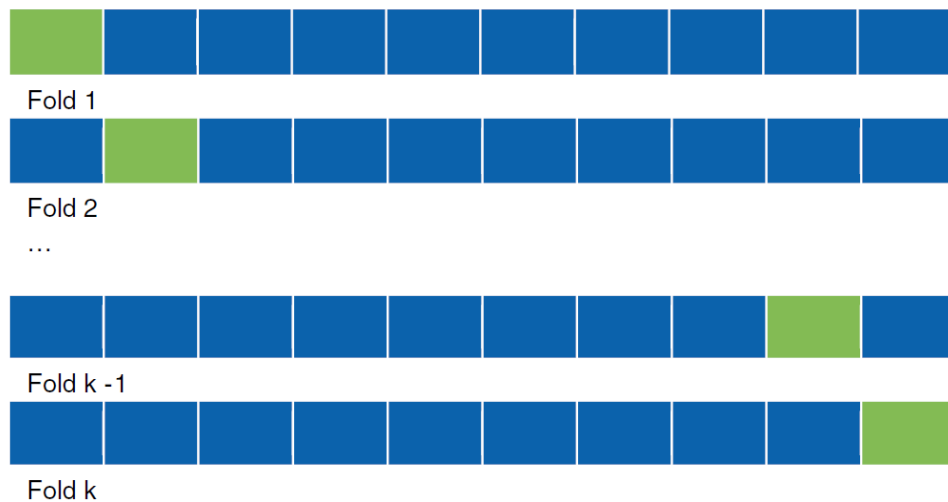
Figure 2-10. K-fold cross-validation adapted from “Building a predictive model of toxicity: methods” [39] by Sunan Cui and et al. in Tiziana Rancati and Claudio Fiorino (eds) in “Modelling radiotherapy side effects: practical applications for planning optimization”, 2019, CRC press and Taylor & Francis Group
