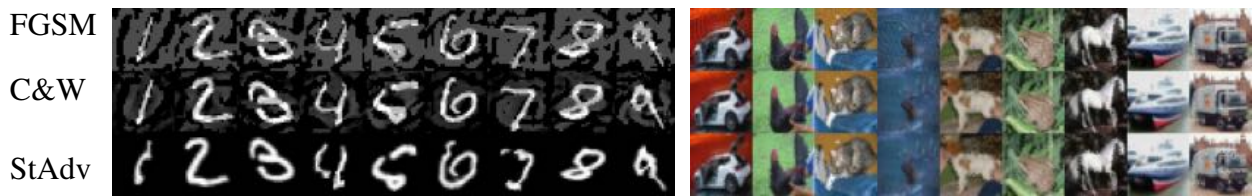
Figure 2.4: Comparison of adversarial examples generated by FGSM, C&W and stAdv. (Left: MNIST, right: CIFAR-10) The target class for MNIST is "0" and "air plane" for CIFAR-10. We generate adversarial examples by FGSM and C&W with perturbation bounded in terms of L_\infty as 0.3 on MNIST and 8 on CIFAR-10.
