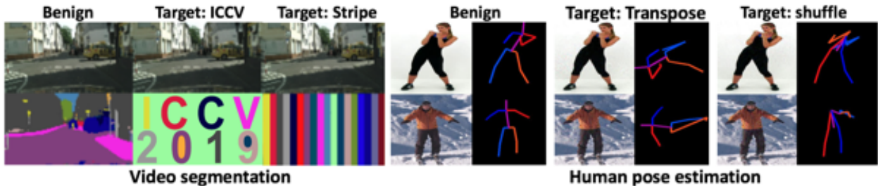
Figure 6.2: Benign and adversarial frames generated on Cityscapes and Davis Challenge 17 dataset for video segmentation and human pose estimation respectively.
