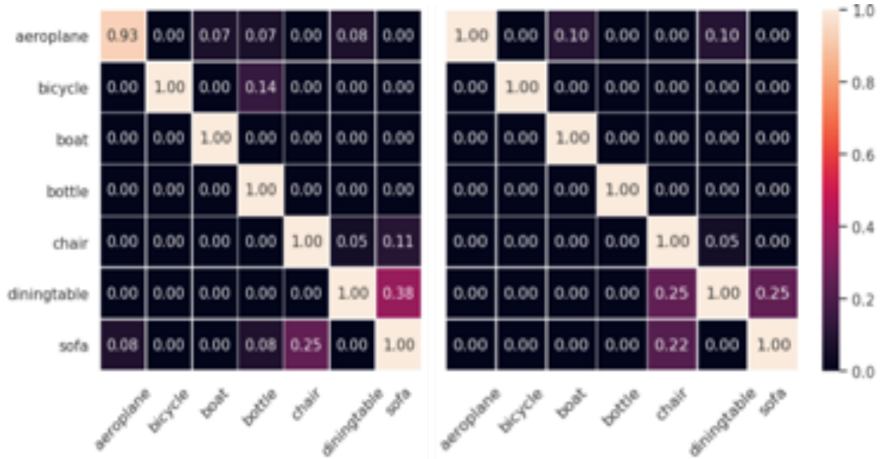
Figure 3.7: Confusion matrices of targeted success rate for evaluating transferability of “adversarial meshes” on different classifiers. Left: DenseNet; right: Inception-v3.
