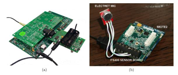
Figure 1.2: (a) Audio sensor mote for acoustic scenes monitoring (2009) (b) TinyEARS (2013).
