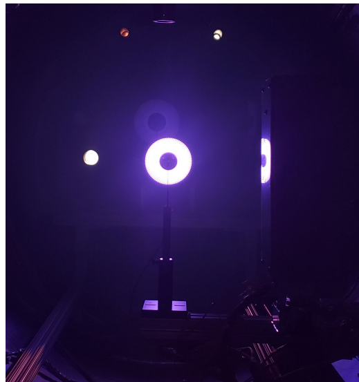
(b) Example of the argon plasma created by the plasma source as viewed from the chamber's view port near the LPs and CubeSat.
