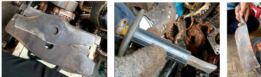
Figure 16: E-waste worker dismantling a stator with a blade and hammer (left). Set of typical tools used to dismantle E-waste (right).
