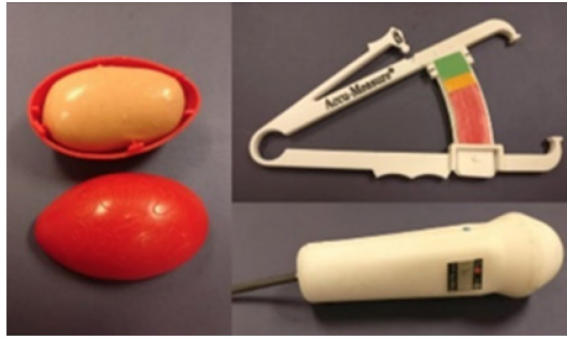
Prototypes for device concept #2: a device to help remove palpable implants
