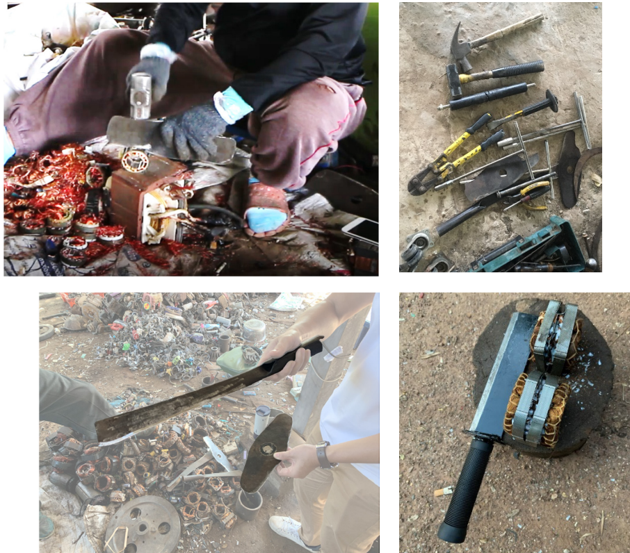
Figure 22: Overview of E-waste tools of interest. Top left: E-waste worker dismantling a stator with a blade and hammer. Top right: Set of typical tools used to dismantle E-waste. Bottom left: Current blades used to dismantle stators. Bottom right: Proposed new tool, locally manufactured, next to a motor.
