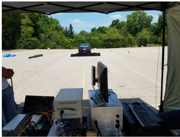
Figure 6.6. The 77 GHz radar measurement scene for a sedan and the coordinate system.
