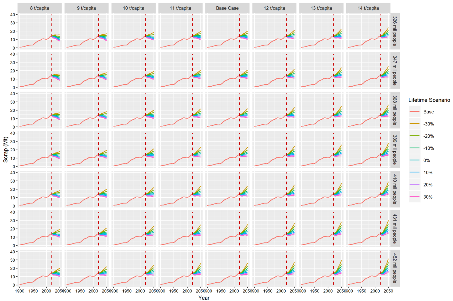
Figure C - 27, U.S. products steel scrap 1900 to 2050 for 2050: stocks per capita ranging from 8 tons/capita to 16 tons/capita (columns), population from 325 to 452 million people (rows), lifespan scenarios ranging from a -30% decrease from average to a 30% increase from average (line color)
