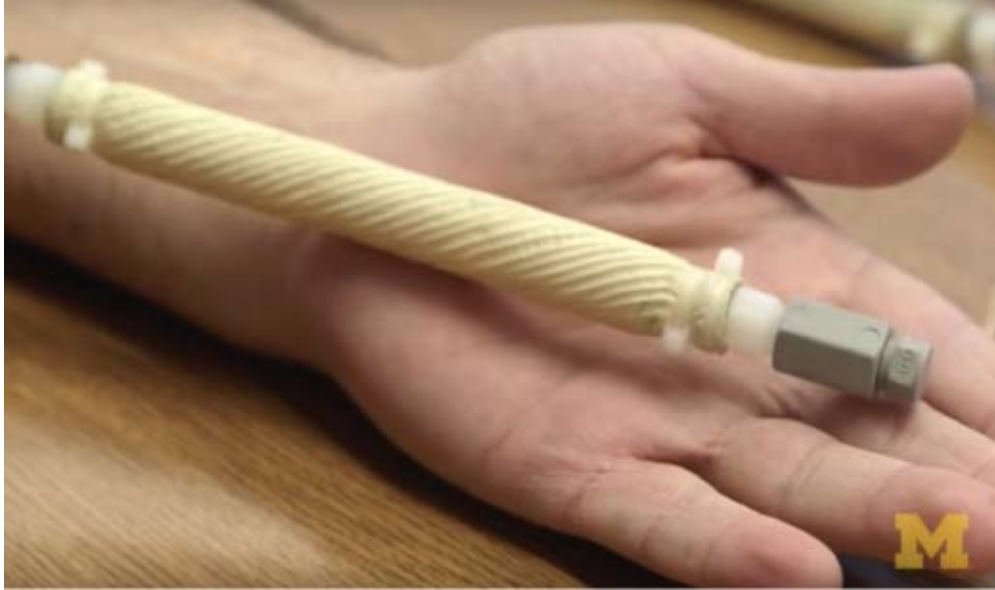
Figure 2.2: A fiber-reinforced elastomeric enclosure (FREE) is a soft fluid-driven actuator composed of an elastomer tube with fibers wound around it to impose deformations such as extension and twisting under an increase in volume.
