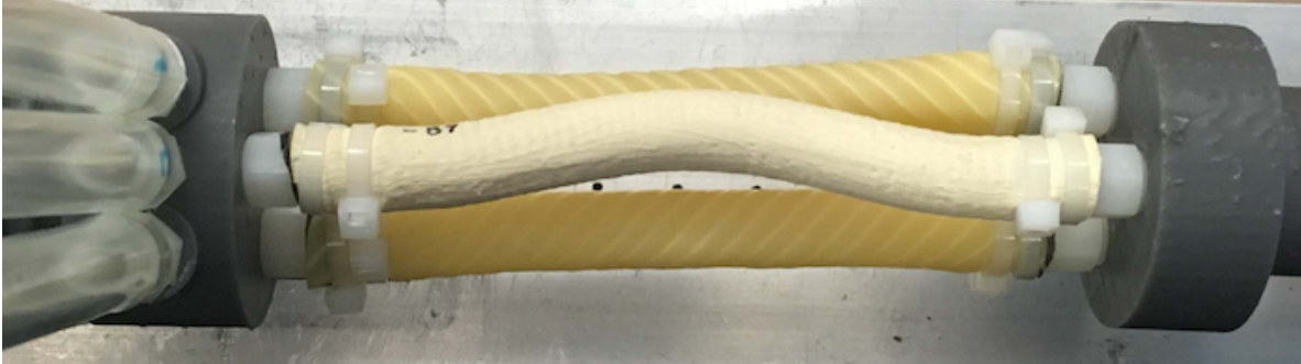
Figure 2.13: At high fluid pressure the FREE with fiber angle of -85^\circ started to buckle. This effect was less pronounced when the system was extended along the z -axis.
