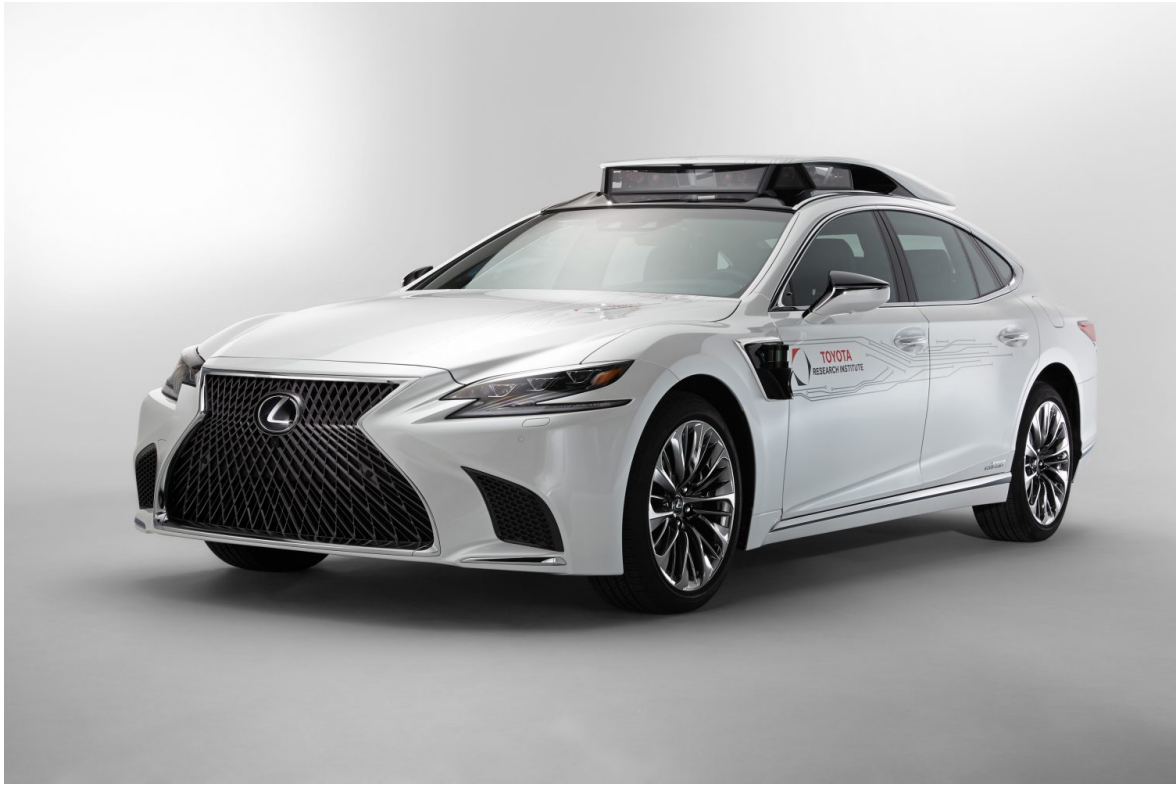
Figure A.1: The Toyota Research Institute test vehicle is a modified Lexus LS 500h with additional sensors for self-driving research.
