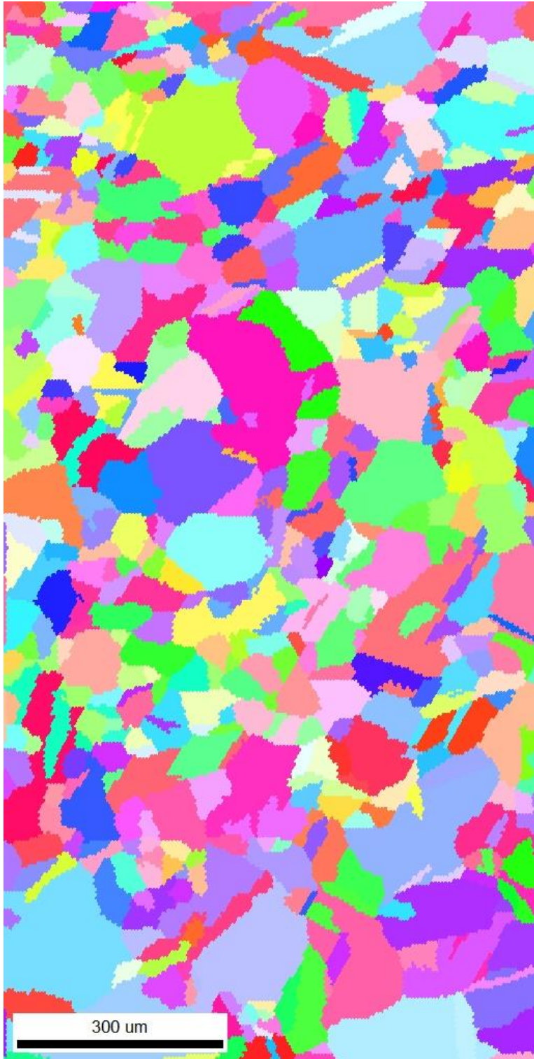
Figure A.28: Inverse pole figure (IPF) taken from BSCC2 Fe21Cr32Ni 5 dpa tensile bar sample OIM region 5 showing grain size and orientation.
