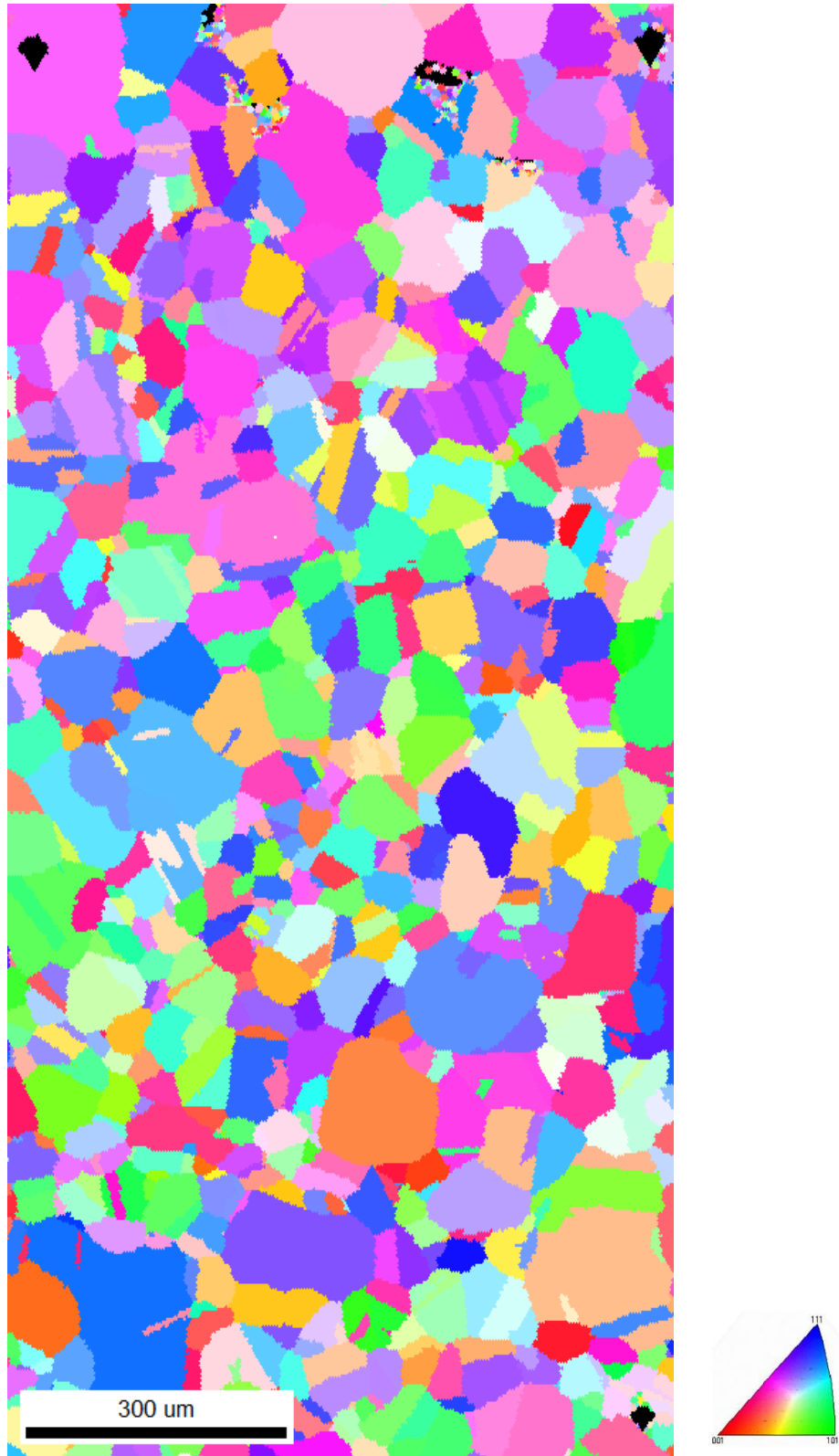
Figure A.541: Inverse pole figure (IPF) taken from ASCC1 Fe13Cr15Ni 0 dpa tensile bar sample OIM region 5 showing grain size and orientation.
