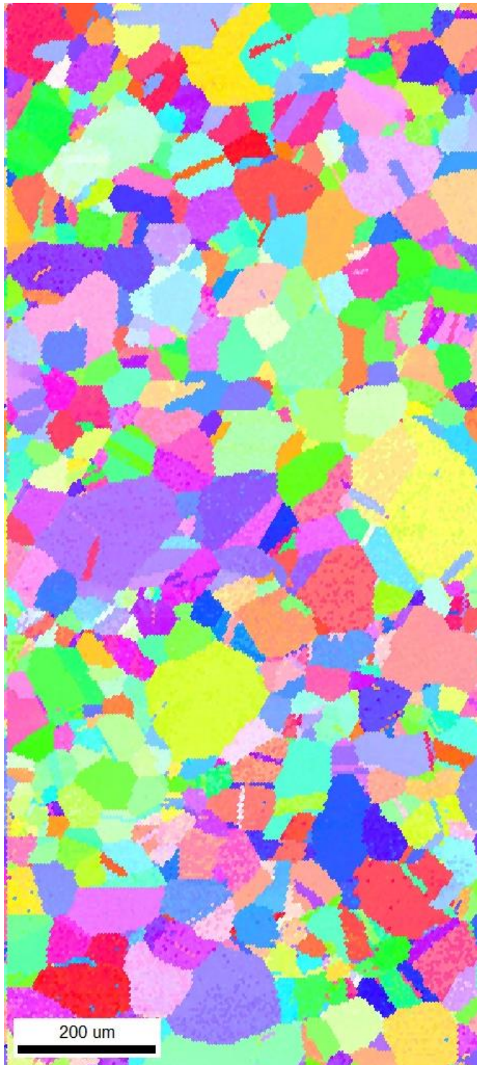
Figure A.1447: Inverse pole figure (IPF) taken from ASCC2 Fe13Cr15Ni 5 dpa tensile bar sample OIM region 7 showing grain size and orientation.
