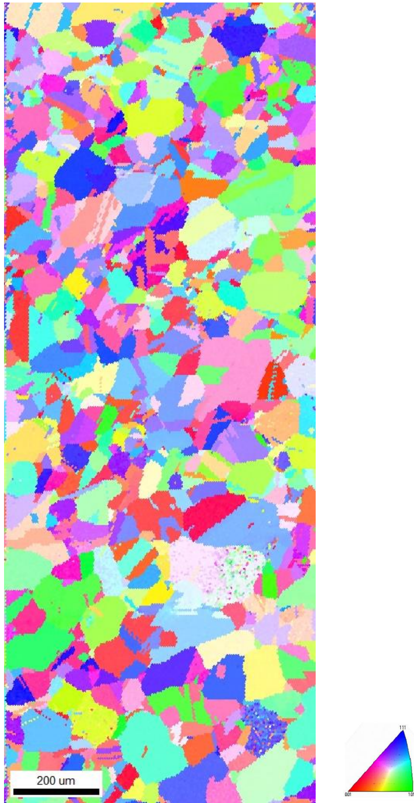
Figure A.24: Inverse pole figure (IPF) taken from BSCC1 Fe21Cr32Ni 0 dpa tensile bar sample OIM region 9 showing grain size and orientation.
