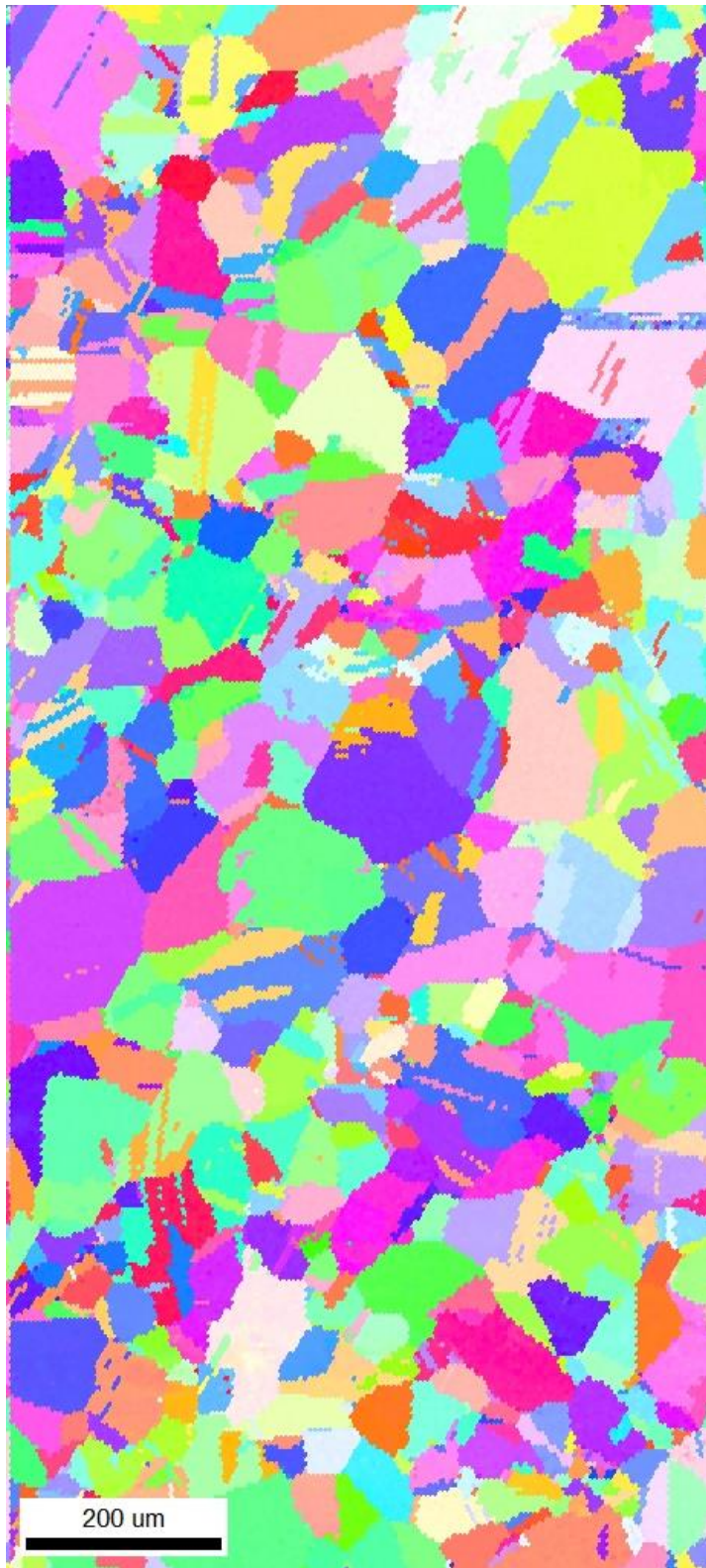
Figure A.2051: Inverse pole figure (IPF) taken from BSCC1 Fe21Cr32Ni 0 dpa tensile bar sample OIM region 5 showing grain size and orientation.
