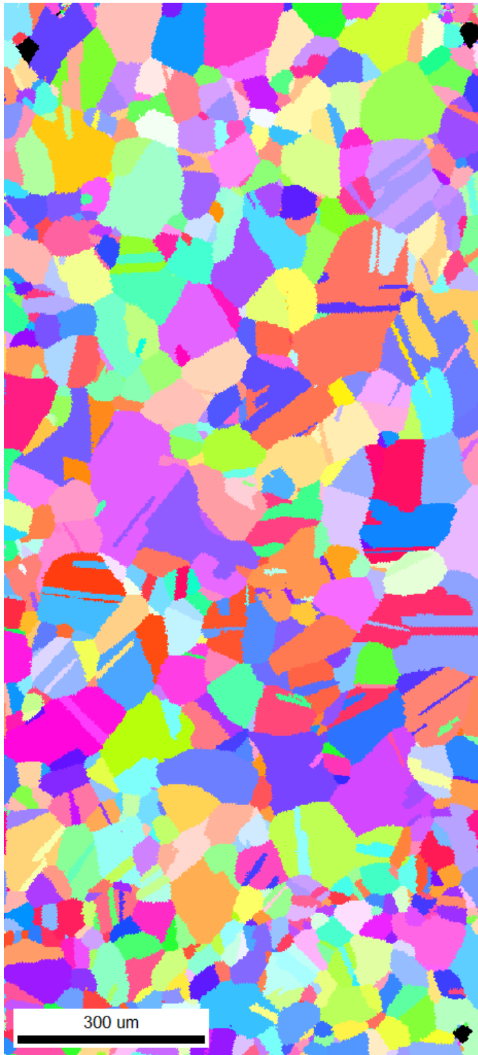
Figure A.3: Inverse pole figure (IPF) taken from ASCC1 Fe13Cr15Ni 0 dpa tensile bar sample OIM region 3 showing grain size and orientation.
