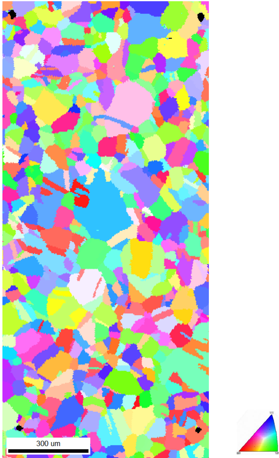
Figure A.239: Inverse pole figure (IPF) taken from ASCC1 Fe13Cr15Ni 0 dpa tensile bar sample OIM region 2 showing grain size and orientation.
