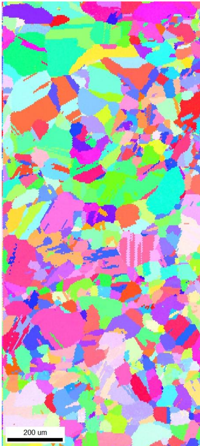
Figure A.23: Inverse pole figure (IPF) taken from BSCC1 Fe21Cr32Ni 0 dpa tensile bar sample OIM region 8 showing grain size and orientation.
