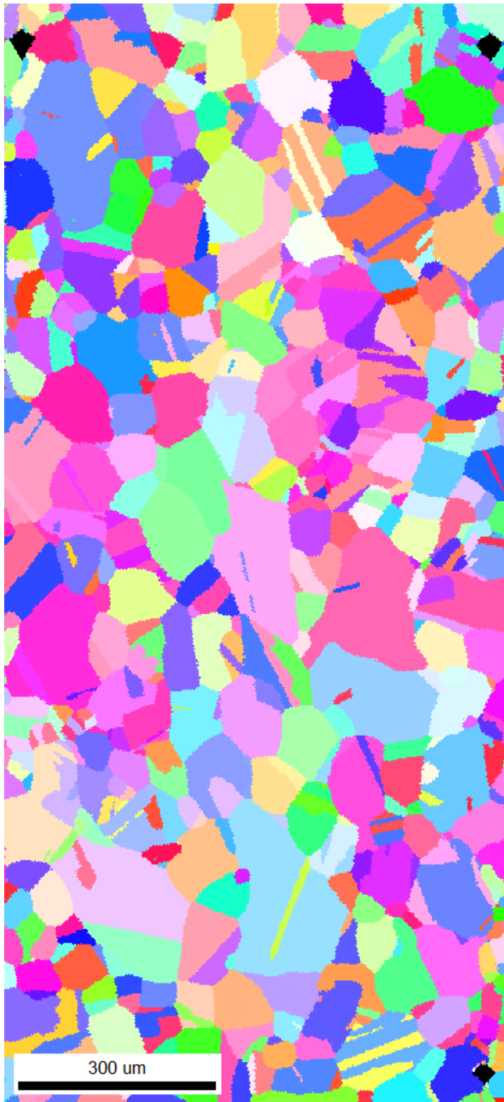
Figure A.44: Inverse pole figure (IPF) taken from ASCC1 Fe13Cr15Ni 0 dpa tensile bar sample OIM region 8 showing grain size and orientation.
