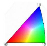
Figure A. 2152: Inverse pole figure (IPF) taken from BSCC1 Fe21Cr32Ni 0 dpa tensile bar sample OIM region 6 showing grain size and orientation.
