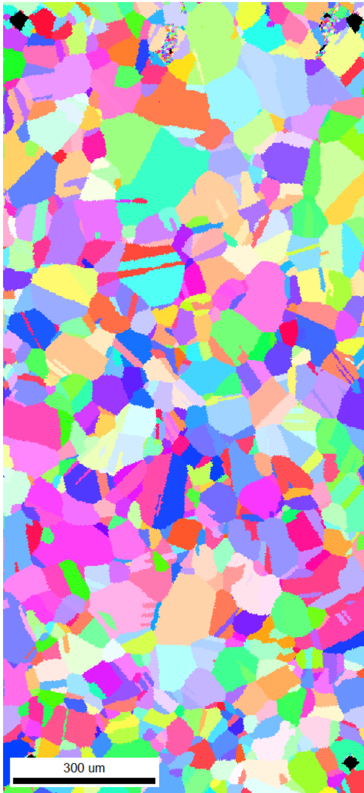
Figure A.743: Inverse pole figure (IPF) taken from ASCC1 Fe13Cr15Ni 0 dpa tensile bar sample OIM region 7 showing grain size and orientation.
