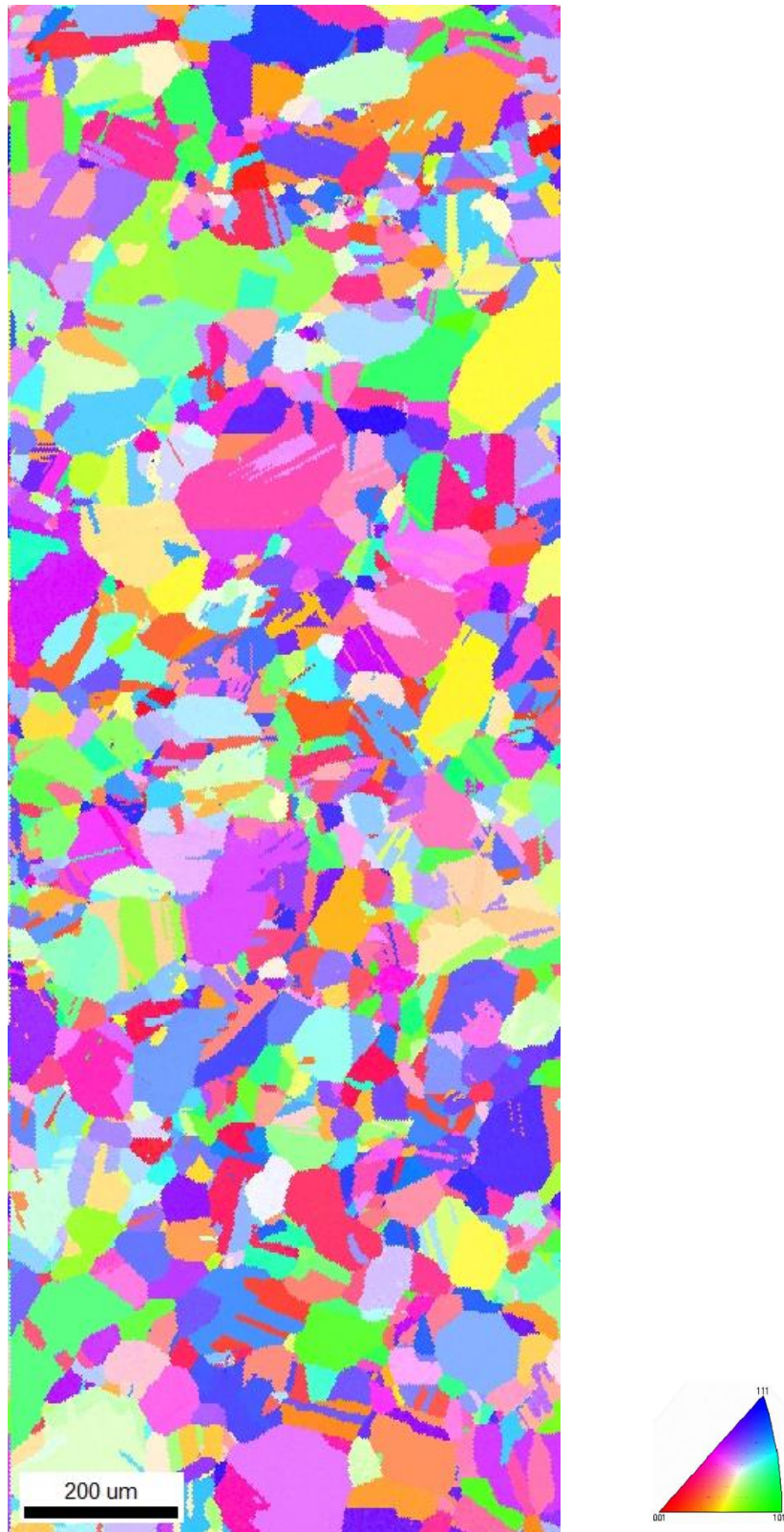
Figure A.26: Inverse pole figure (IPF) taken from BSCC1 Fe21Cr32Ni 0 dpa tensile bar sample OIM region 1 showing grain size and orientation.
