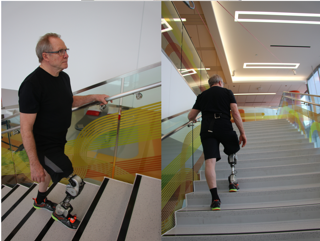
Figure B.6: Walking up stairs with the OSL at the Shirley Ryan AbilityLab.
