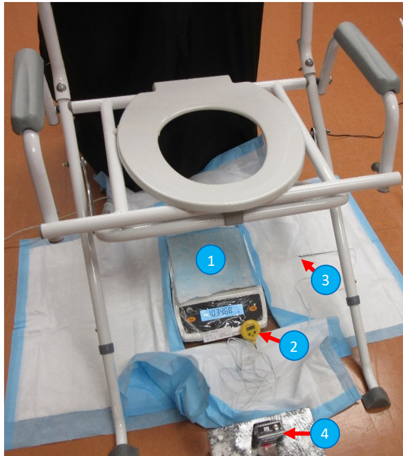
Figure 40. Commode setup above the precision balance (1) where the urine collection container (not shown in the figure) was placed. A thermometer (2) also recorded the temperature of the voided urine into the container with its probe (3) when placed in the collection container. A camera (4) was used to record bypass leakages occurred during the micturition.
