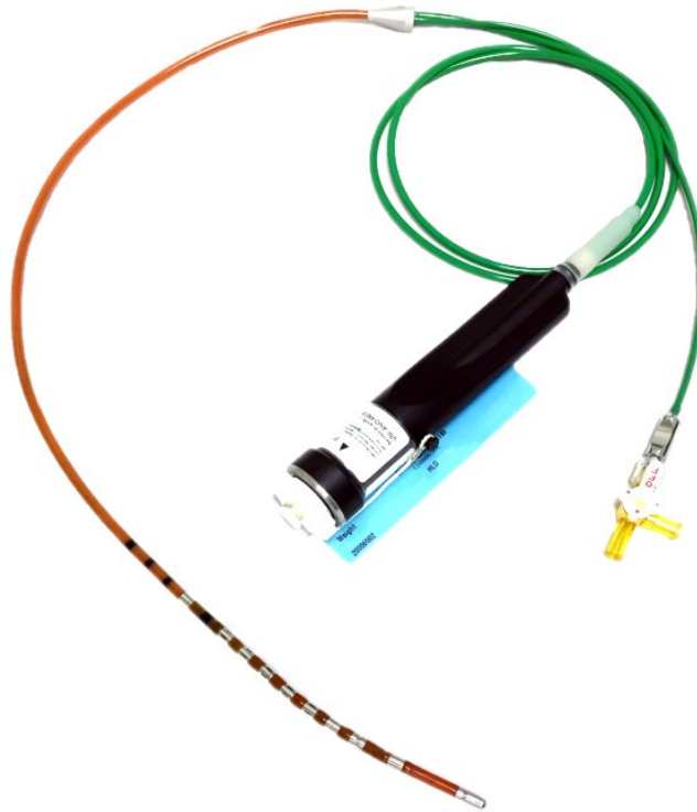
Figure 48. HR-ARM probe Sandhill Scientific® HR-ARM system (Denver, CO, USA) comprised of an array of pressure sensors on a 4 mm diameter catheter with internal air tubing to inflate the balloon (not installed in this picture) on the tip of the catheter.
