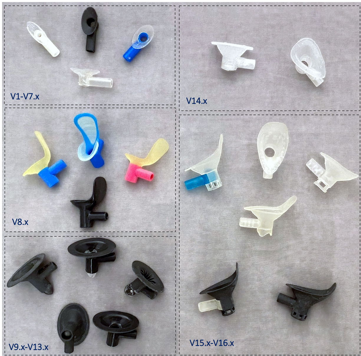
Figure 27. Examples of rapid prototyped PUF housings; the first PUF housing (V1) designed to be integrated with a modified incontinence patch. Blue and pink PUF housings in the upper left box were 3D printed from multiple stiffness materials in a single printing process. b) PUF housings (V9.x-V12.x) made from Flexible SLA resin (Formlabs®); the stiffness of the walls can be controlled by adjusting the thickness. PUF V14.x were made with 3D printed housings and soft over-molded biocompatible silicones. A dispersion silicone was used to cover typical printed parts to ensure biocompatibility.
