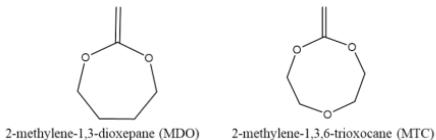
Figure 1.3: Cyclic ketene acetal (CKA) monomer rings for MDO and MTC.
