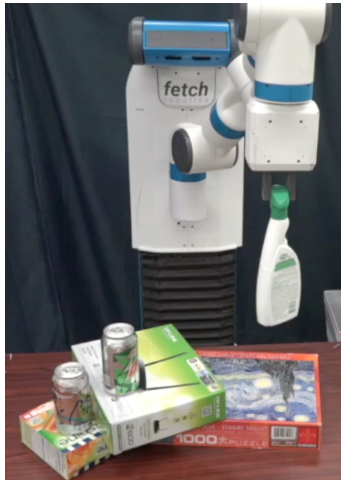
Figure 4.7: An example case study where the Fetch Robot successfully picked up a spray bottle based on an Amazon Mechanical Turk worker’s annotation using EURECA.
