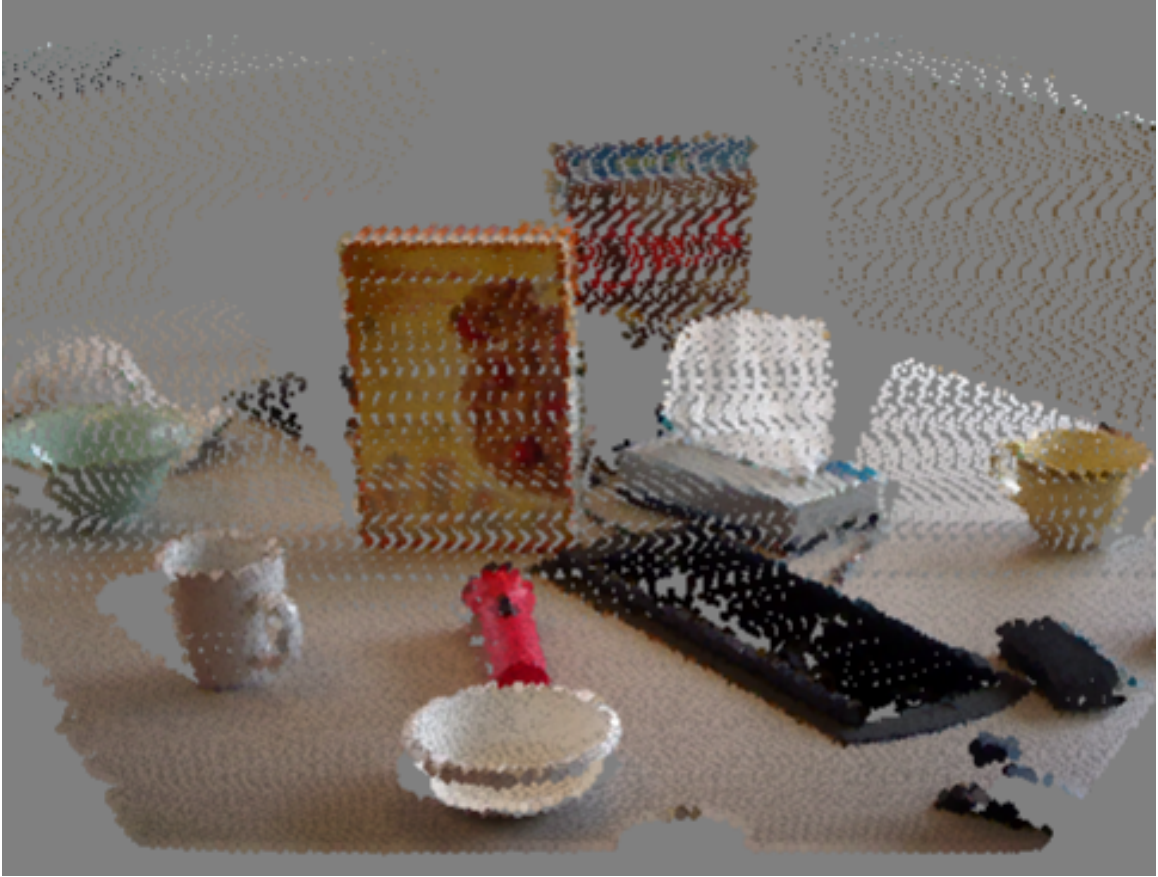
Figure 4.8: An colored (RGB) version of the point cloud that is seen in Figure 4.2. Even though RGB helps to visually differentiate between the objects, we did not see any significant improvements in annotation speed and accuracy.
