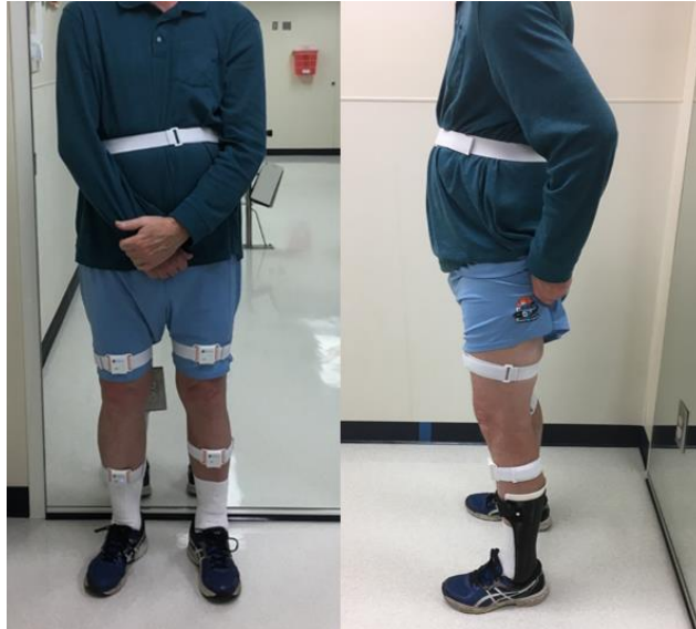
Figure 3-5: IMU attachment for the LEGSys™: one IMU on each thigh, one on each shank, and one on the lower back trunk.
