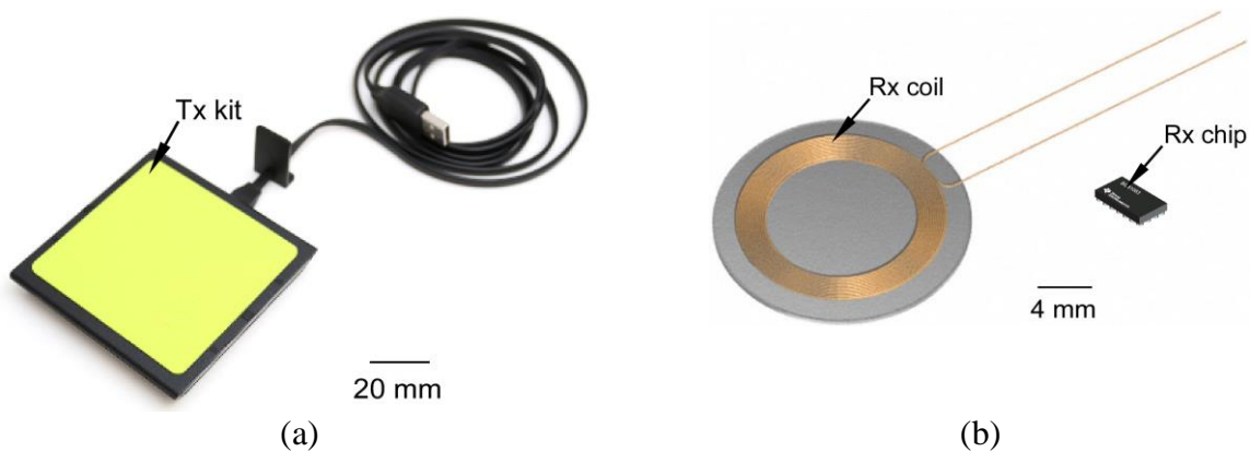
Figure 3.3: (a) Transmitter kit and (b) receiver coil and chip for wireless charging of ELM7.
