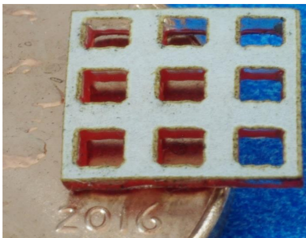
Figure 5.5: Photo of perforations in acrylic adhesive tape.
