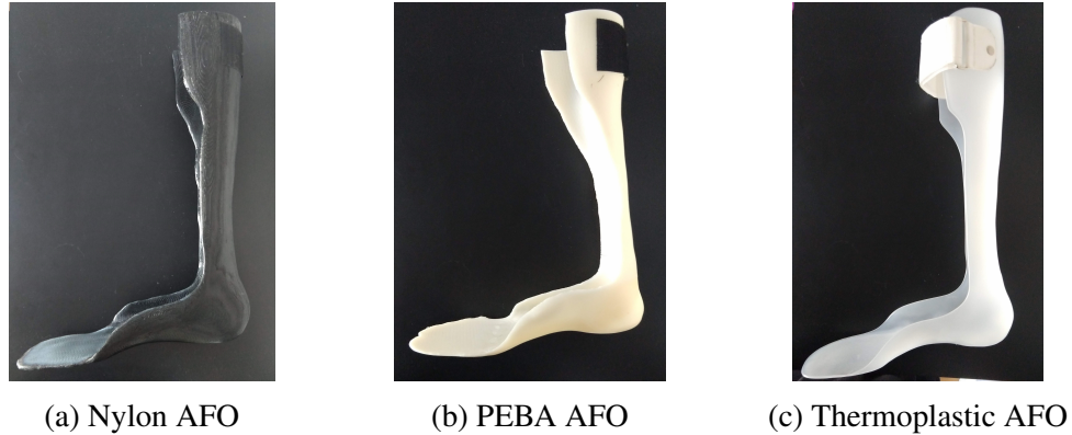
Figure 4.1: The three AFOs used in this study. The nylon, PEBA, and thermoplastic AFOs had wall thicknesses of 7.5, 3.6, and 3.5 mm, foot lengths of 27.0, 28.0 and 27.0 cm, and heights of 39.0, 36.0, and 41.5 cm, respectively.
