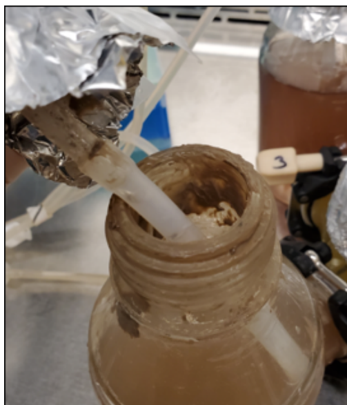
(a) Image of biofilm formation and accumulation in the 500 mL A. vinelandii partition
