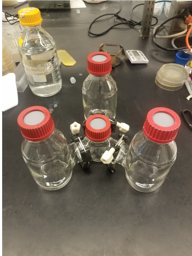
Figure B.3: Depiction of specialty separated tripartite culture vessel. The three main chambers (top, left, and right) are modified 500 mL Pyrex bottles. The middle chamber is a modified 100 mL Pyrex bottle. Flanges tighten the glass bottle connection, which consists of two plastic rings with a rubber washer between.
