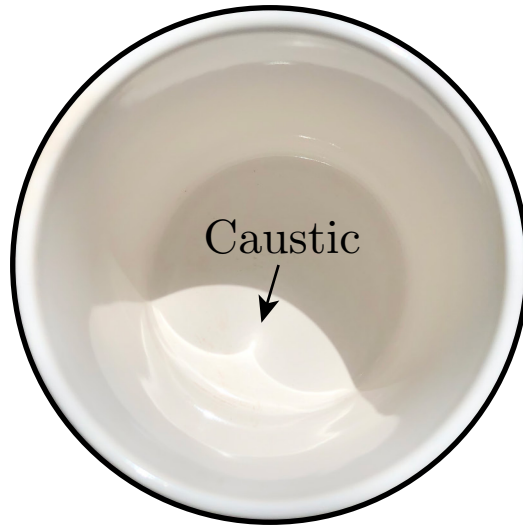
Figure 2.1: An optical caustic formed by the cylindrical reflecting surface of a coffee cup.
