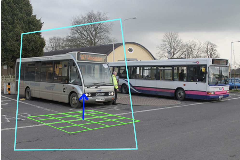
Figure 4.3: Surface normal annotation UI. The surface normal is visualized as a blue arrow originating from a green grid, rendered in perspective projection according to the known focal length.
