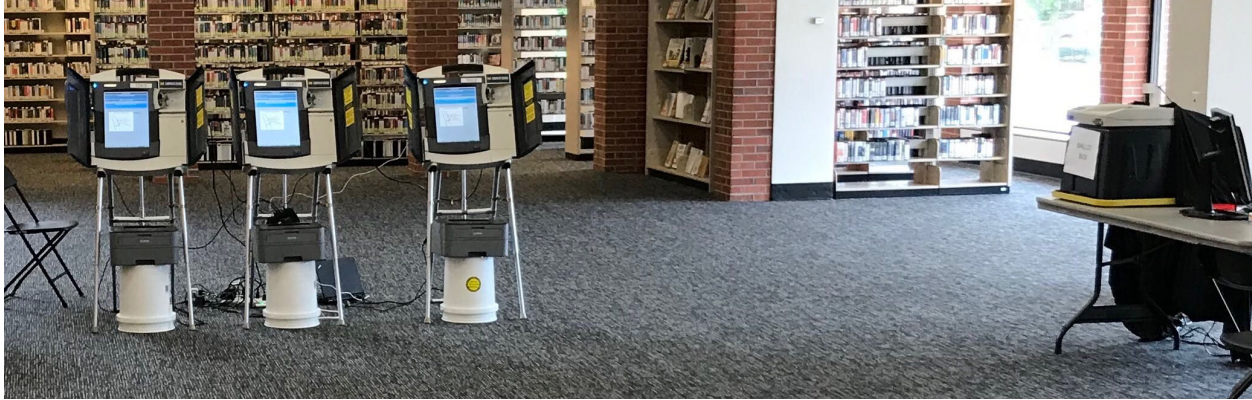
Figure 4.1: Polling Place Setup . We established mock polling places at two public libraries in Ann Arbor, Michigan, with three BMDs ( left ) and an optical scanner and ballot box ( right ). Library visitors were invited to participate in a study about a new kind of election technology. The BMDs were DRE voting machines that we modified to function as malicious ballot marking devices.
