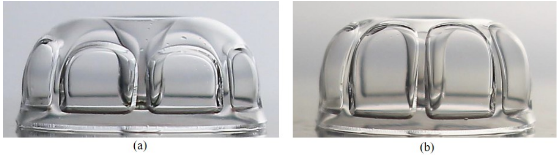
Figure 2.36: Shells with different aspect ratio of thin windows fabricated by changing dimensions of etched features on the patterned substrate.
