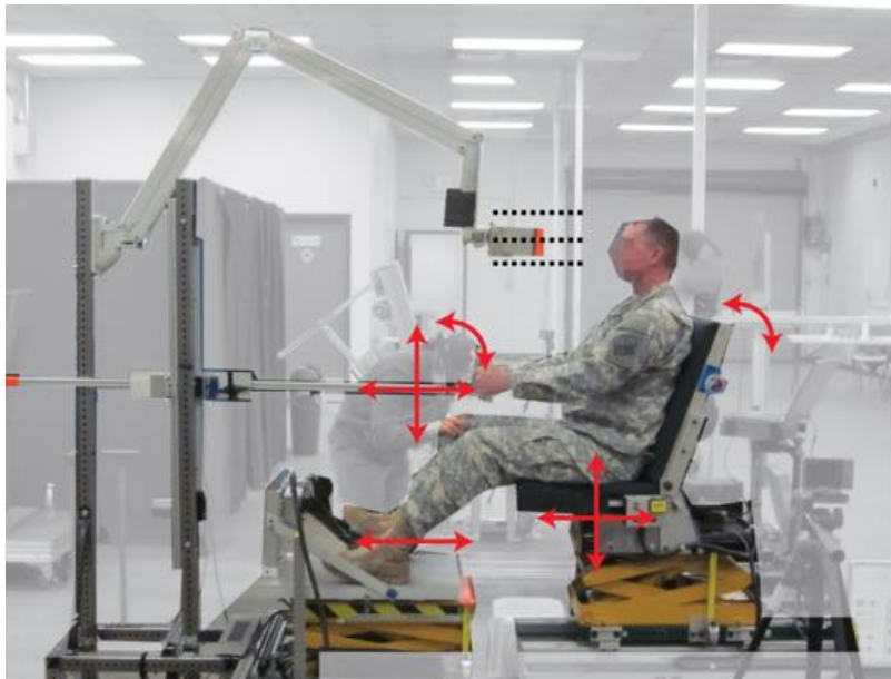
Figure 9. FEP mockup. Red arrows show motorized adjustment ranges available to participant.
