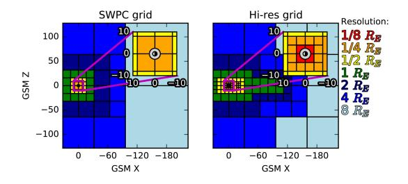
Figure 2. X-Z cuts showing cell sizes in the two MHD grids (reproduced from Haiducek et al., 2017). (Left) The grid used for the *SWPC* configuration (minimum cell size of 0.25  $R_E$ ). (Right) The higher-resolution grid used for the *Hi-Res SWPC* configuration (minimum cell size of 0.125  $R_E$ )
