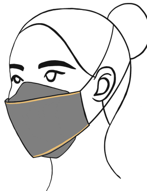
Figure 8. The figure below depicts where the metal wire was added to the structure of the mask as a result of the comfortability tests. This addition of wire is meant to be molded away from the user's face to create space between the user's mouth and the mask. The space created is expected to help the breathability of the mask.
