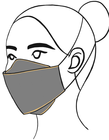
Figure 10. This figure shows a drawing of where the wire is sewn into the outer cloth layer. The orange line in the picture represents the wire.
