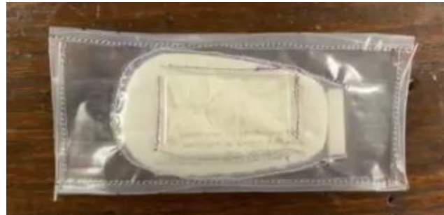
Figure 16. In this figure you can see the N95 filter inserted into the plastic layer which is completed in Step 5 of assembling the mask.
