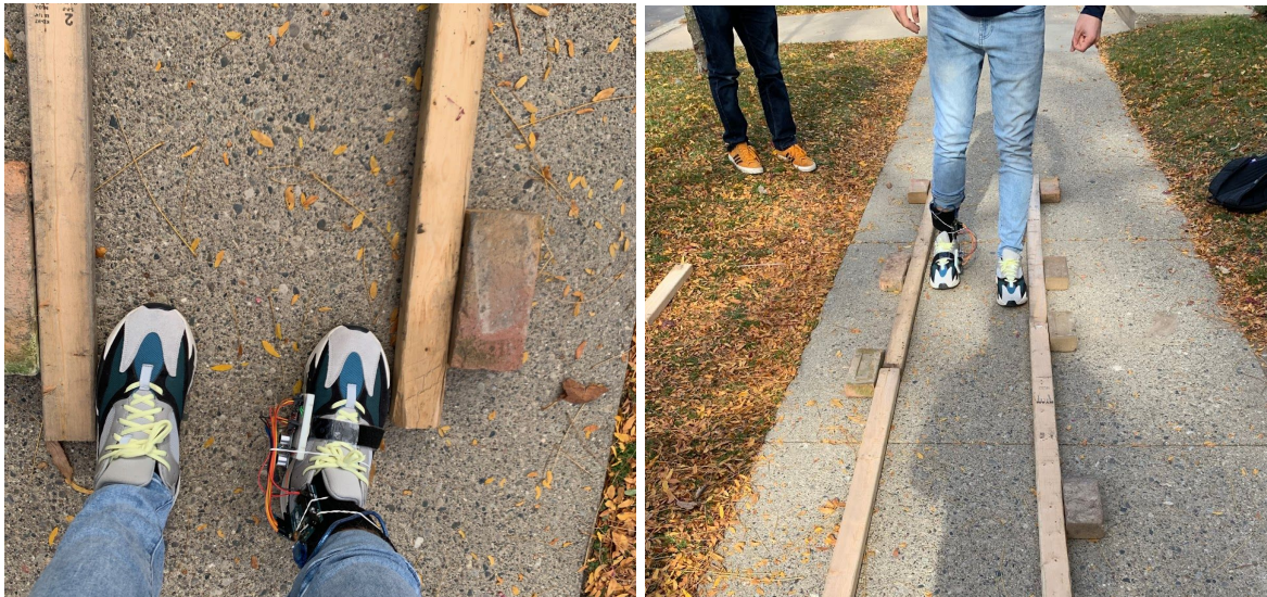
Figures 24: The second walking test was conducted using rails made from 2" x 3" pieces of wood and supported by bricks. These rails aligned the subject's step width to a distance of about 6.5 inches
