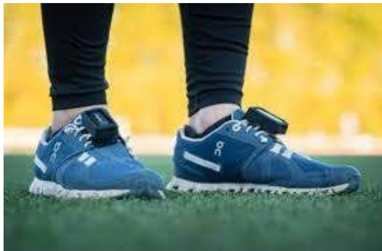
Figure 6: Two IMU data loggers attached to the laces of somebody's shoes [Stammel, 10]
