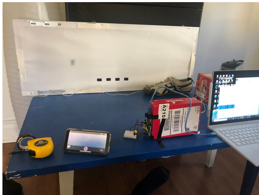
Figure 15: Dynamic Velocity Testing Experimental Setup
