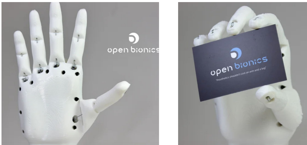
Figure 19. The Ada Hand V1.1 by Open Bionics. The neutral finger positions (left) and all five fingers being actuated to grip a business card (right).
