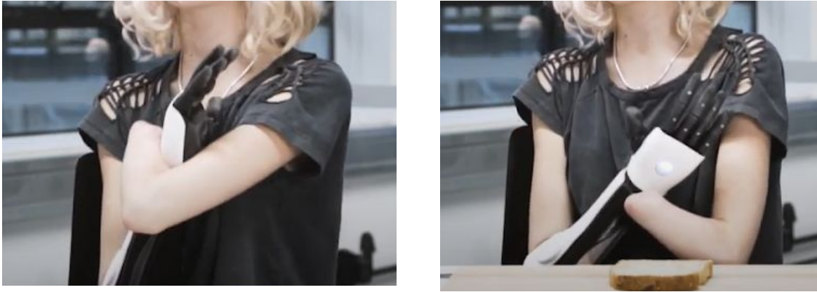
Figure 6. Left to right shows the change in orientation of the Hero Arm Prosthetic. This operation is manual and requires direct user input. [12]
