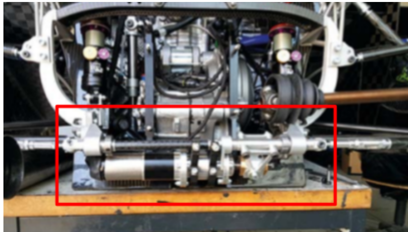
Figure 8: TU Graz 2019 Rear Steer System. Single steering rack is similar to our concept 1
