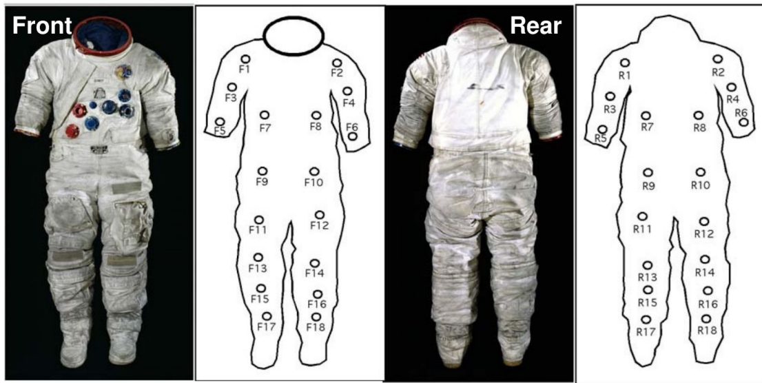
Figure 6. Standard imaging of anterior and posterior positions of Apollo 17 EVA spacesuit. Areas of highest lunar dust concentration are shown as dark grey patches near the leg, upper torso, and forearm areas. Bare schematics with ovals represent lunar dust sampling locations for tape extraction procedure.
