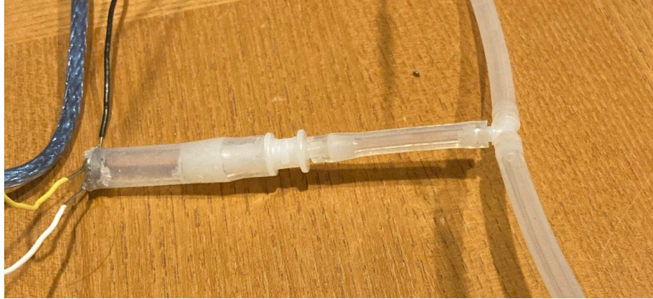
Figure 31. T-shaped connector connecting the pressure sensor, suction cup, and vacuum pump
