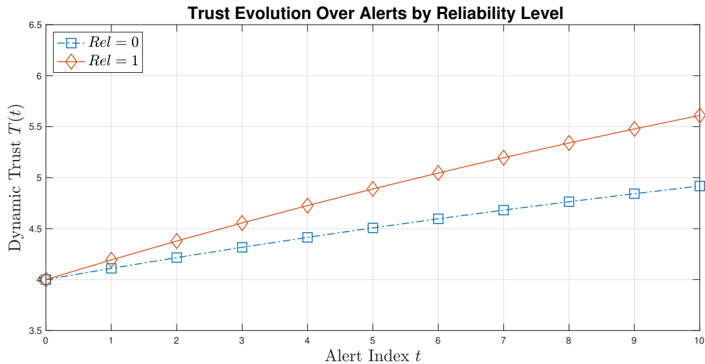
Figure 6. Curves illustrate the simulation of the model represented by Equation (5). We chose T(0) = 4 for both conditions to better compare the results. When Rel = 1 (i.e., when participants were using a reliable ADS), trust increased faster than when Rel = 0 (i.e., when participants were using an unreliable ADS). For both curves, Vis = 0 .
